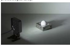
Natural light distribution when illuminating a wider work area with an equivalent to a 40W incandescent bulb with 550 lumens.
